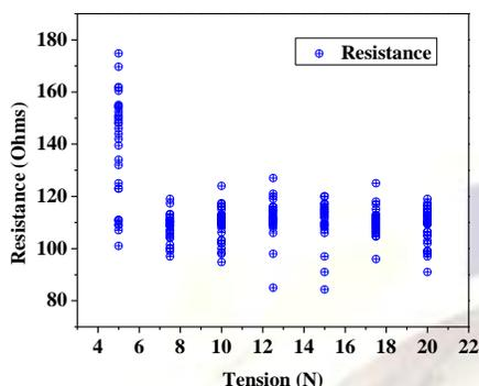
Figure 4 Resistance vs. tension plot.
