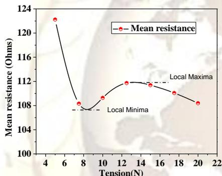
Figure 5(a) Mean resistance vs. tension.
