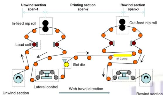
Figure 1(b) Schematic representation of slot die coating system
