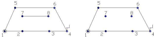
Figure 2. (a) Dependent link connection. (b) Independent link connection
