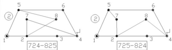
Figure 6. The concept of Isomorphic graphs for independent link connection
