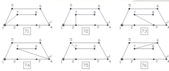
Figure 10. Available arrangements for connecting link 7 with original links in dependent link connection
