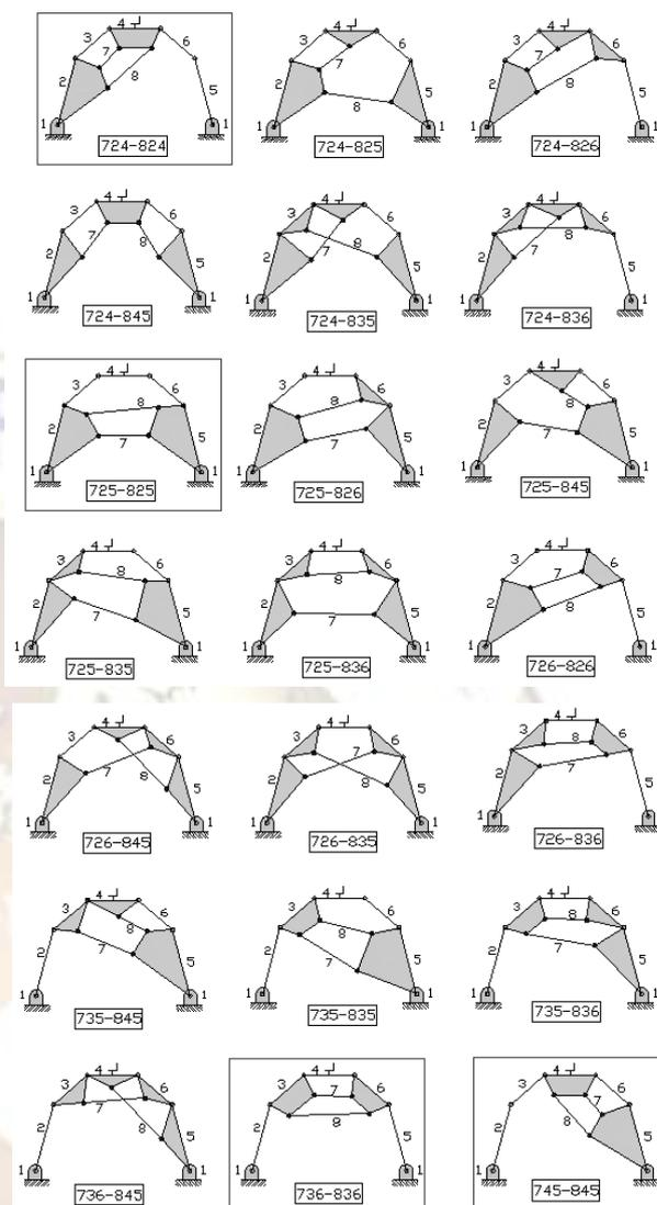
Figure (9) Corresponding linkage diagram for enumeration results of independent link connection
