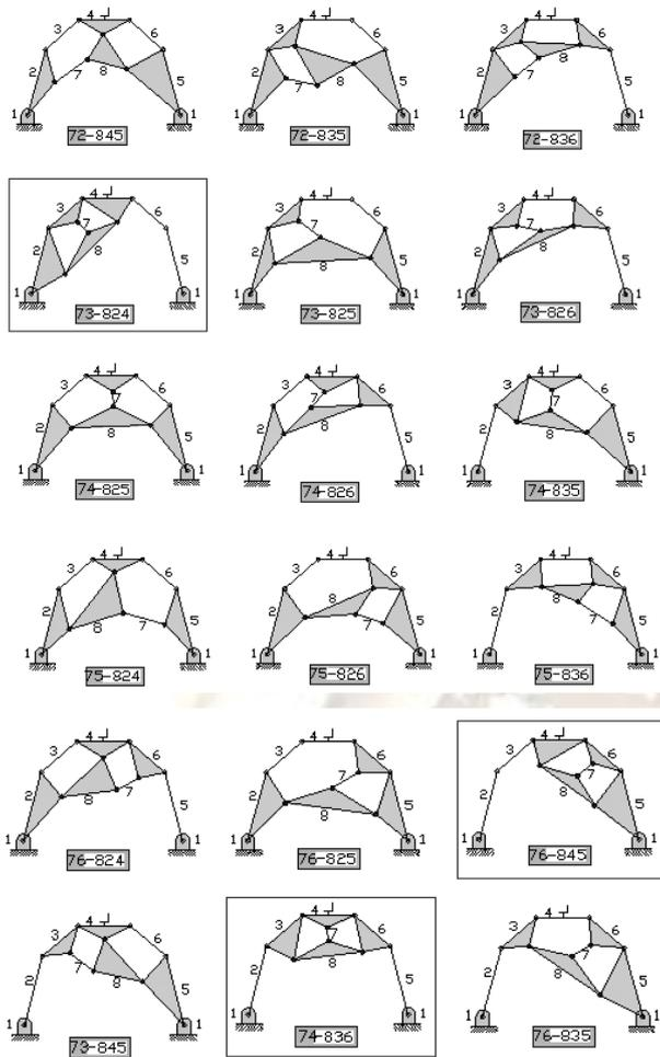
Figure 13. Corresponding linkage diagram for enumeration results of independent link connection
