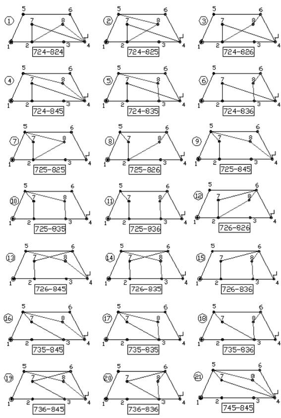
Figure 7. Non isomorphic graphs for independent link connection
