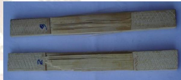
Fig. 14. Mode of failure on Layered Laminate Bamboo Composites.
