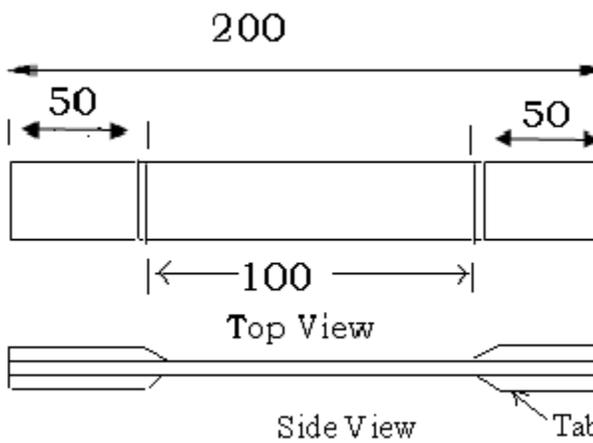
Fig.3. Sketch of lamina Specimens with tab.
