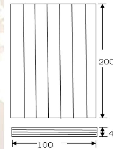
Fig.5. The bamboo epoxy layered laminated bamboo composite.
