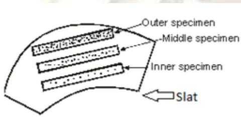
Fig. 2. Location of lamina specimens on slats.
