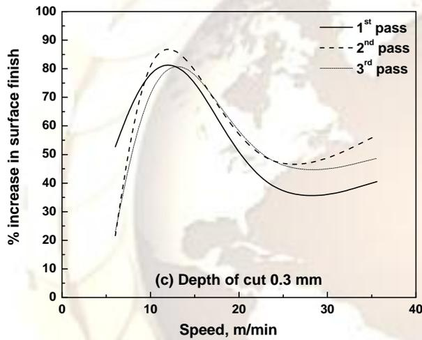
Fig. 3: Variation of burnishing speed with % increase in surface finish for different passes with different depth of cut for AA6061 alloy.
