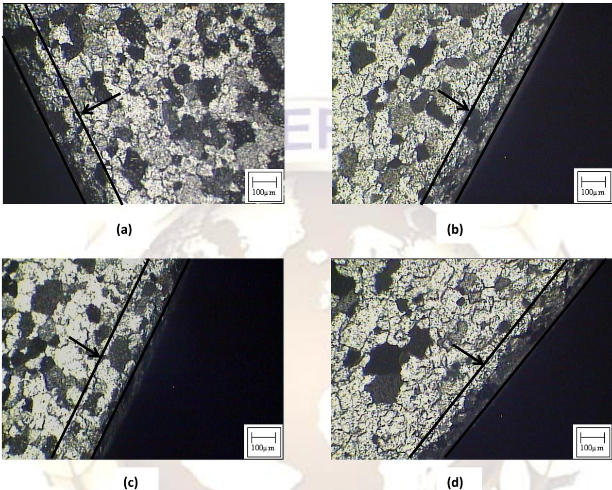
**Fig. 5: Optical micrograph of AA6061 alloy showing the depth of burnishing in (a) Unburnished (b) burnished – 1<sup>st</sup> pass (c) burnished – 2<sup>nd</sup> pass (d) burnished – 3<sup>rd</sup> pass condition.**
