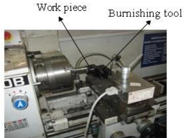
**Fig. 2: Burnishing setup used in the present study.**
