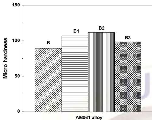
**Fig. 7: Correlation of surface micro-hardness with burnishing parameters**
