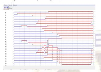
Fig.7.wave form for 8 bit multiplier using body biasing
