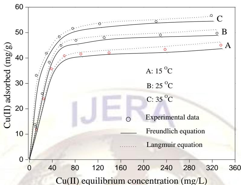
**Figure 1. Cu(II) adsorption isotherm.**
