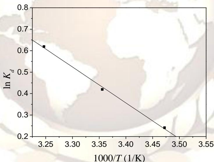
Figure 2. A plot of  $\ln K_d$  against  $1/T$  for Cu(II) adsorption by rice husk.
