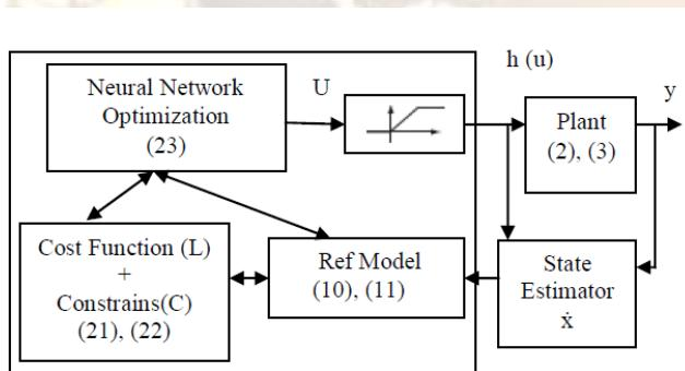
Fig. 3. Block diagram of NMPC with neural network optimization
