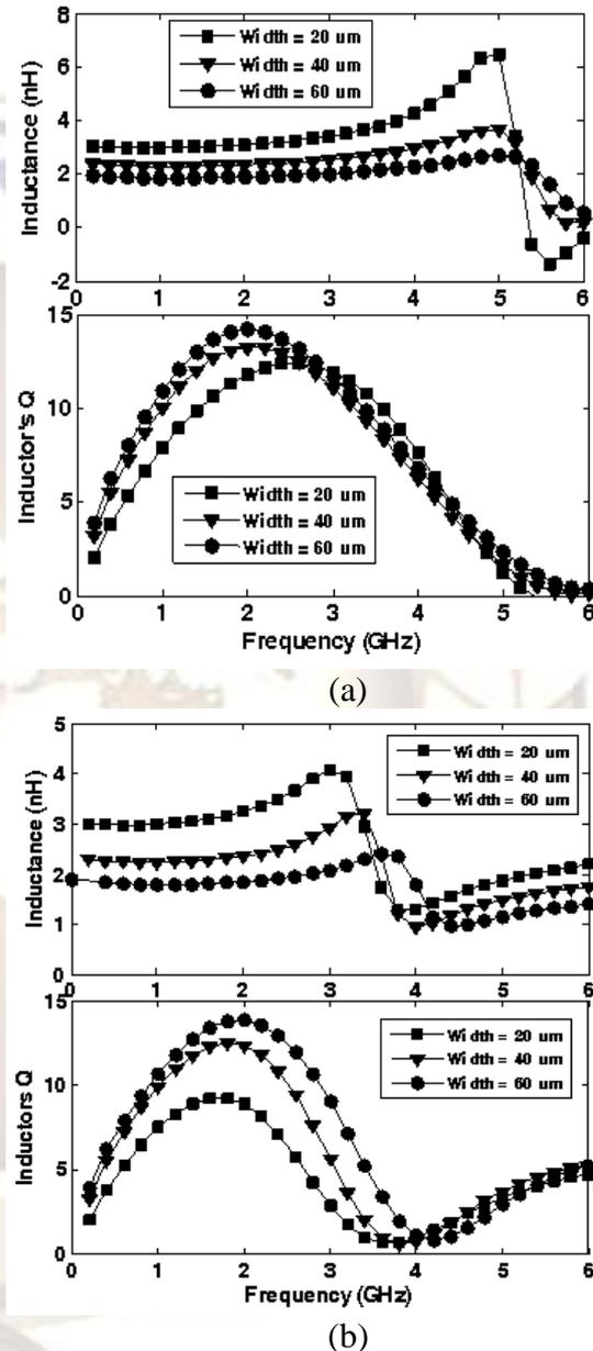
Fig. 5. Inductance and Q-factor of the proposed network with different metal width for power combiner with (a) two transformer or Fig.1a (b) three transformer and third transformer is single-turn inductor or Fig.1b
