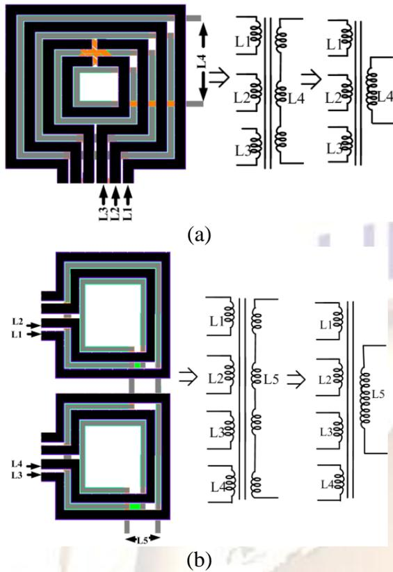
Fig.2. Proposed transformer network and equivalent circuit as power combiner with (a) three transformer and third transformer is two-turn inductor (b) four transformers
