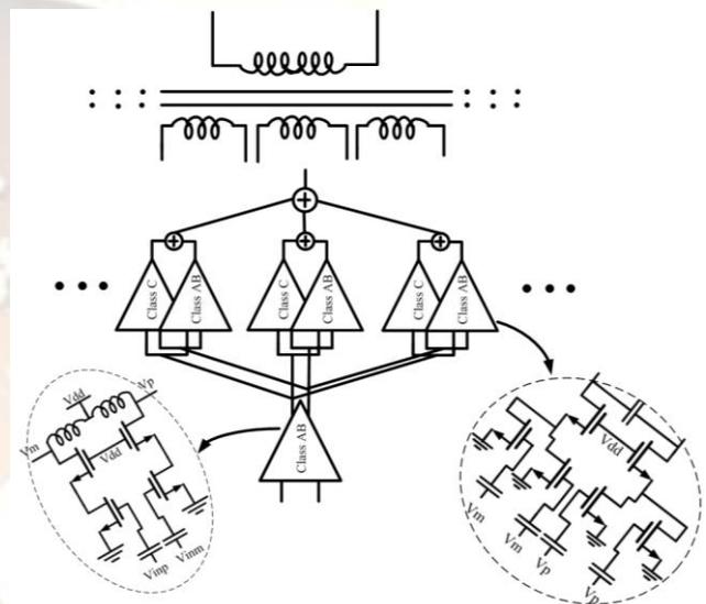
Fig. 7. Circuit schematics of the Power Amplifier
