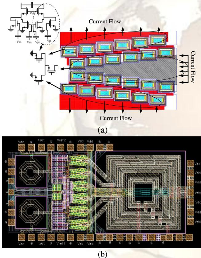
Fig. 8. (a) Layout diagram of Power Stage (b) Layout diagram of Power Amplifier
