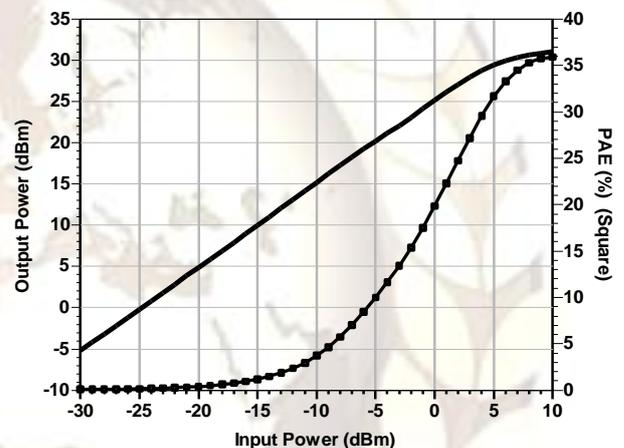
Fig. 9. Output power and PAE simulation result
