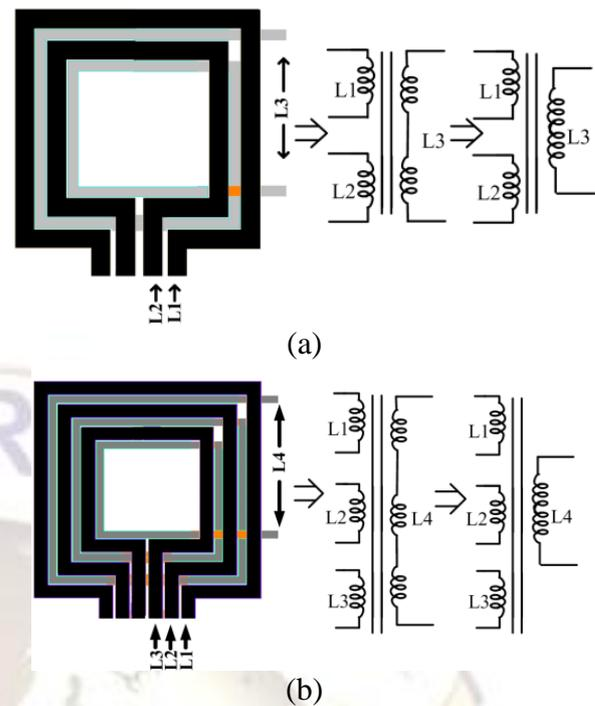
Fig.1. Proposed transformer network and equivalent circuit as power combiner with (a) two transformers (b) three transformer and third transformer is single-turn inductor
