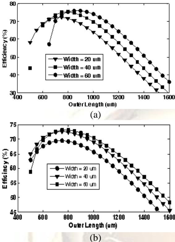
Fig. 4. Efficiency versus OD and metal width for power combiner with (a) three transformers and third transformer is two-turn inductor or Fig.2a (b) four transformers or Fig.2b
