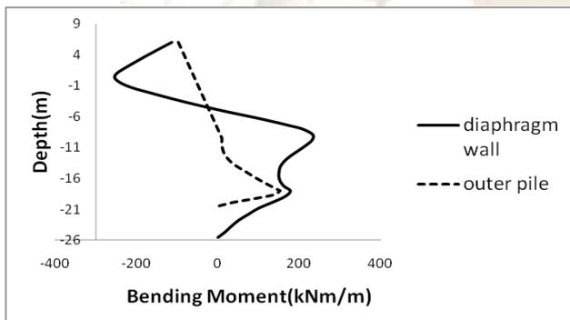
Fig.8 Comparison of bending moments of the diaphragm wall and outer pile due to seismic effects
