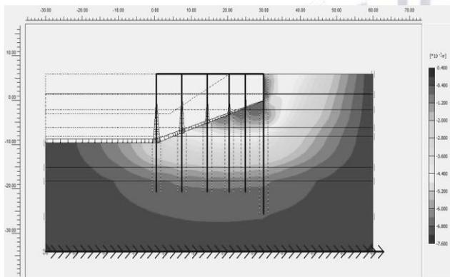
Fig.3 Extreme total displacement in static analysis
