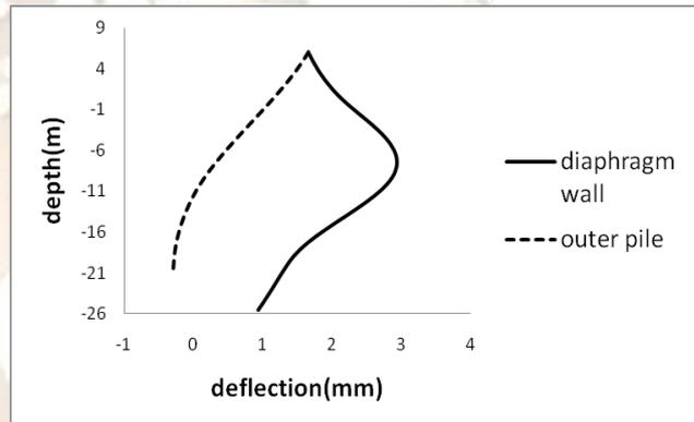
Fig. 6 Comparison of displacements of the outer pile and diaphragm wall under seismic effects
