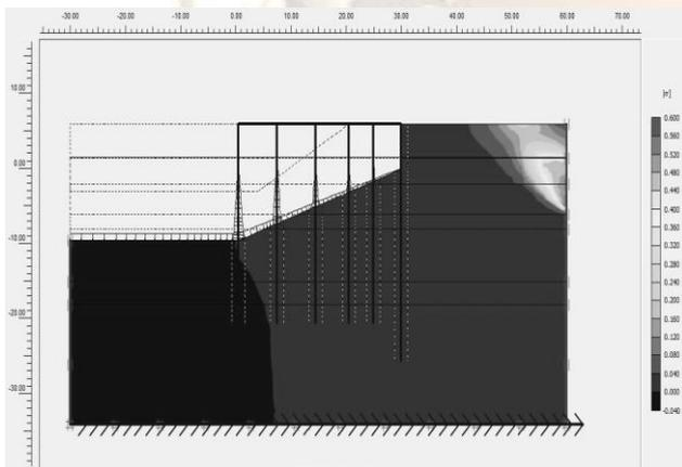
Fig.4 Extreme total displacement in dynamic analysis
