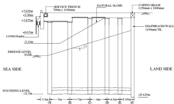
Fig. 1 Typical cross section of the berth
