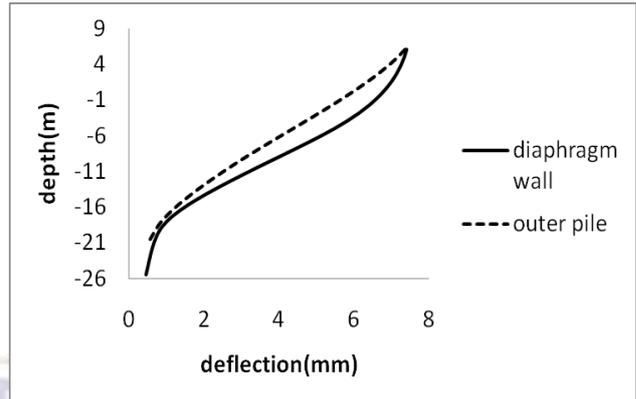
Fig.5 Comparison of displacements of the diaphragm wall and pile after -9.5m dredging
