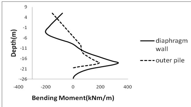
Fig.7 Comparison of bending moments of the diaphragm wall and outer pile due to dredging effects
