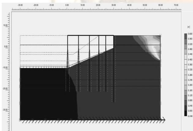
Fig.4 Extreme total displacement in dynamic analysis
