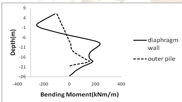
Fig.8 Comparison of bending moments of the diaphragm wall and outer pile due to seismic effects
