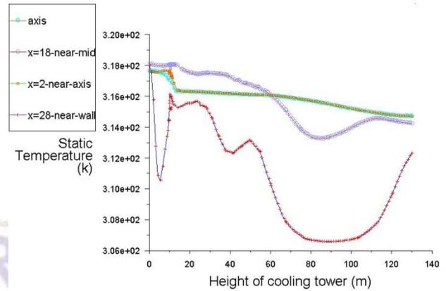
To investigate thermal performance of tower with increase in height three line have been drawn as near axis ,near wall and between axis and wall. Temperature is having its high value in middle line and lower near the wall. The graph shows at very near to wall its value is very low around 307 k and out let axis having highest value of temperature.
