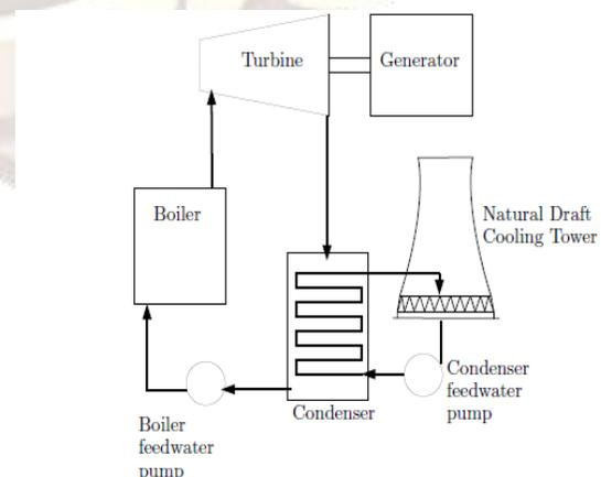
Figure 1. Power plant cycle with cooling tower
