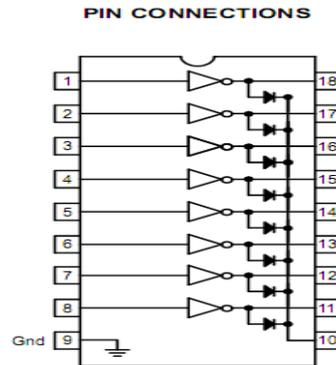
The eight NPN Darlington connected transistors in this family of arrays are ideally suited for interfacing between low logic level digital circuitry (such as TTL, CMOS or PMOS/NMOS) and the higher current/voltage requirements of lamps, relays, printer hammers or other similar loads for a broad range of computer, industrial, and consumer applications. All devices feature open-collector outputs and freewheeling clamp diodes for transient suppression.
