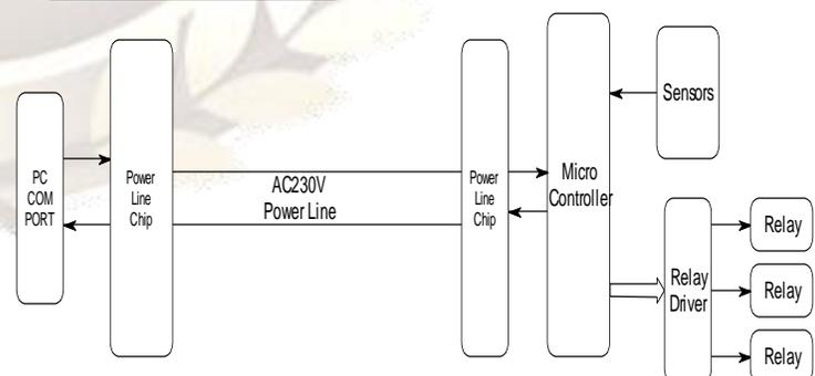
**3.1 Functional Description:-** In this Project the data is being transferred over AC line from PC communication port, which is encoded and decoded by PLC chips. The received information signal is then send to the microcontroller and according to the
