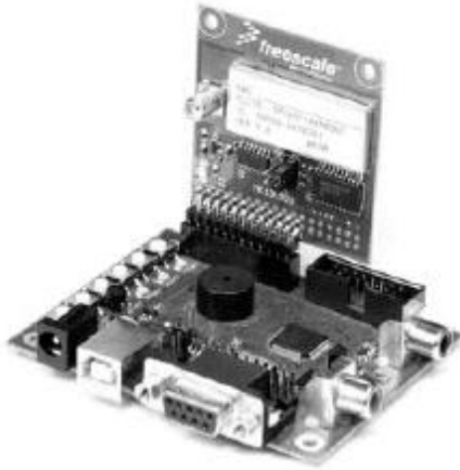
Fig. 6 The DEMC ARM BOARD with LPC2138 microcontroller with inserted Freescale RF board
