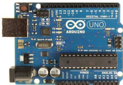
Arduino has 14 input/output pins on one side (labeled 0 through 13) and 6 input/output pins
