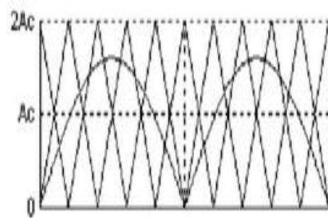
**Fig 2: Carrier arrangement for APOD technique**
