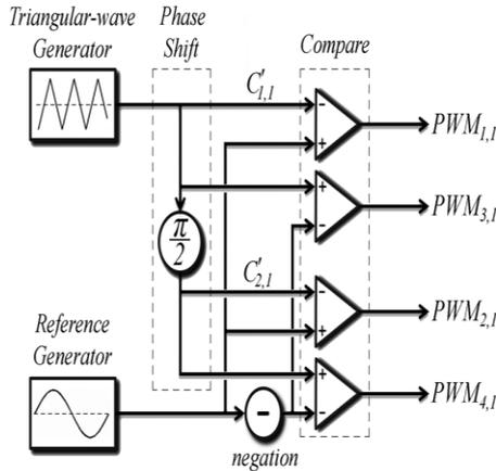
Fig 3: Block diagram for (five-level) PSC
