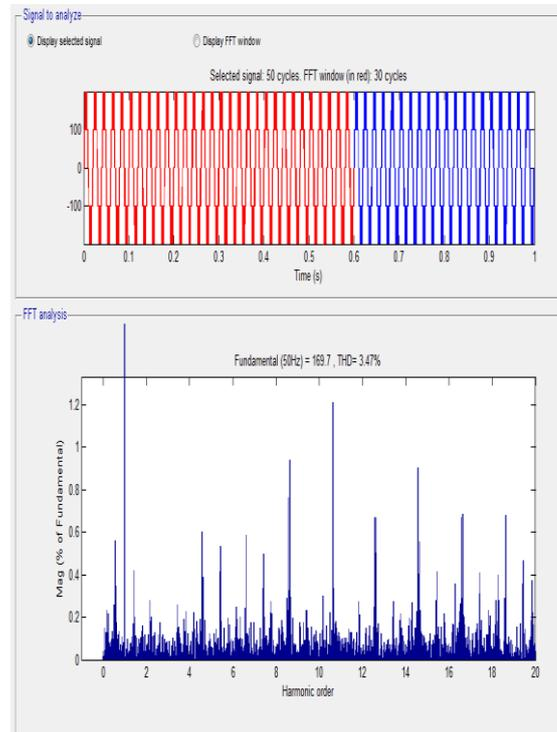
Fig 15 : Output voltage and Harmonic Analysis wave forms.
