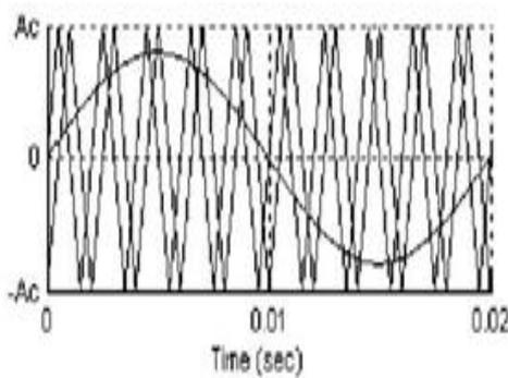
Fig 4: result for (five-level) PSC operation
