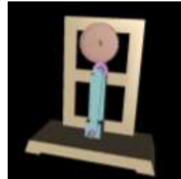
Fig. 15: Crank and Slotted Lever Mechanism
