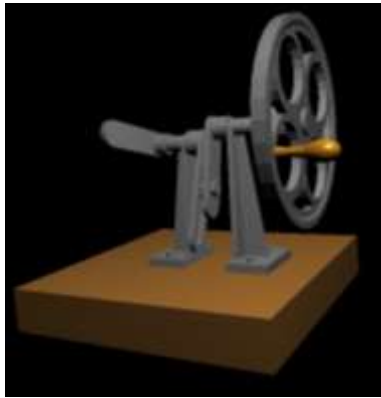
Fig. 1: Withworth Quick Return Mechanism
