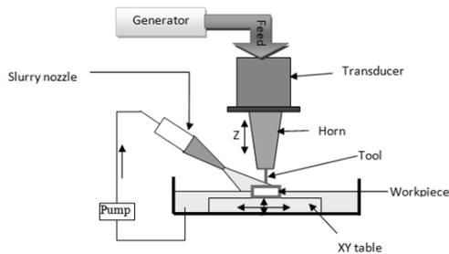
Fig 1: Schematic of A Micro USD Process
