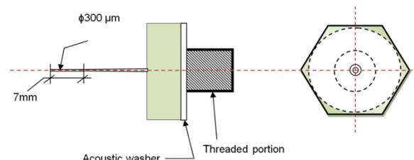
Figure 3: Schematic Of A Typical Micro Tool
