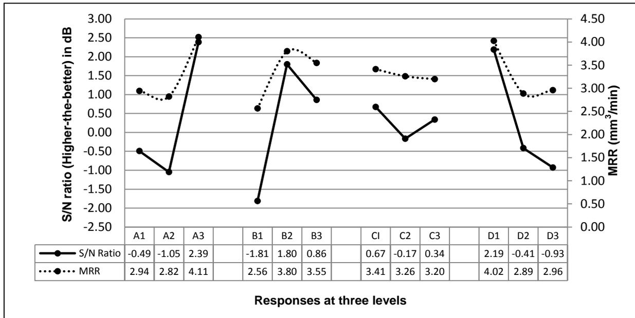
Figure 4 Effect Of Process Parameters On Mrr Raw Data And S/N
