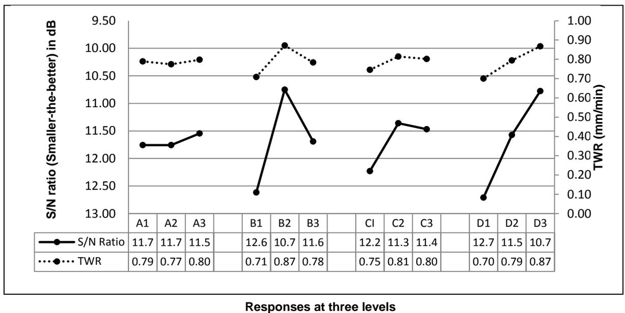
Figure 5 Effect Of Process Parameters on TWR Raw Data And S/N
