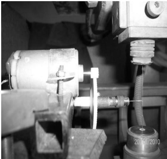
Figure 2: The Wedg Set-Up Used For Making Microtools
