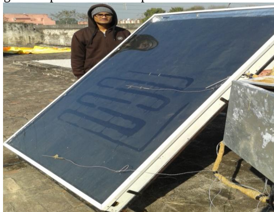
Fig. 2: Flat-Plate Collector Used in Experiment
