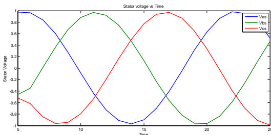
Fig 5.1 Stator Open Circuit Voltages
