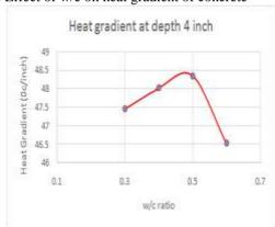
This figure illustrates that 50% w/c ratio gives the highest heat gradient.
