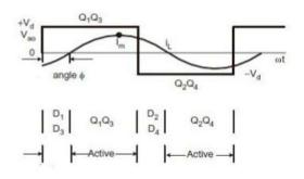
Fig.5 Load voltage and current waveform
