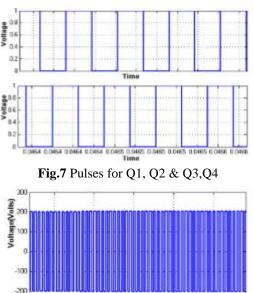
Fig.8 Inverter output voltage
