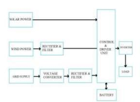
Fig.1 Block diagram of hybrid energy system
