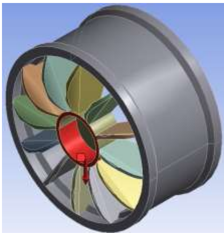
Fig.7 Load application and direction
