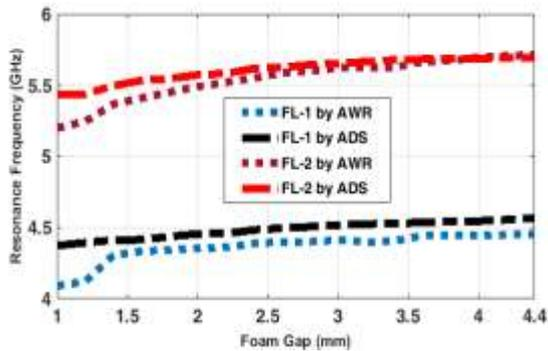
Figure 2: Variation of the resonance frequency with Height of Substrate foam gap
