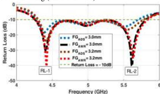
Figure4: Better of Power reflection coefficient (S11) for two different values of foam gap height
