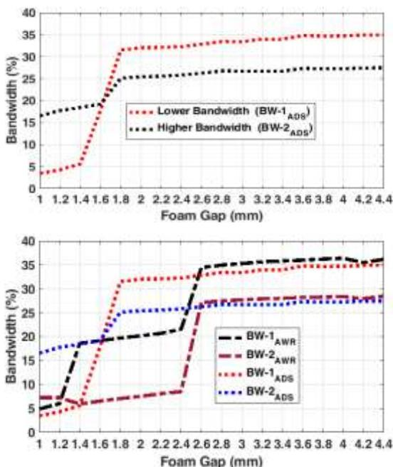
Figure 8: Variation Bandwidth with Height of Substrate foam gap.
