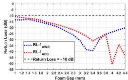
Figure 6: Variation of the Reflection Coefficient (S11) with Height of Substrate foam gap (AWR & ADS).
