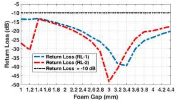
Figure 5: Variation of the Reflection Coefficient (S11) with Height of Substrate foam gap (AWR)
