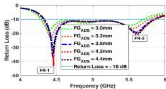
Figure 3: Power reflection coefficient (S11) and resonance frequency for different values of foam gap height.
