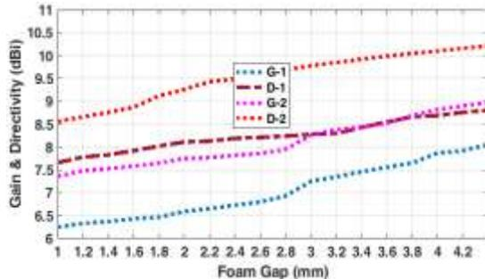
Figure 7: Variation Gain and Directivity with Height of Substrate foam gap.
