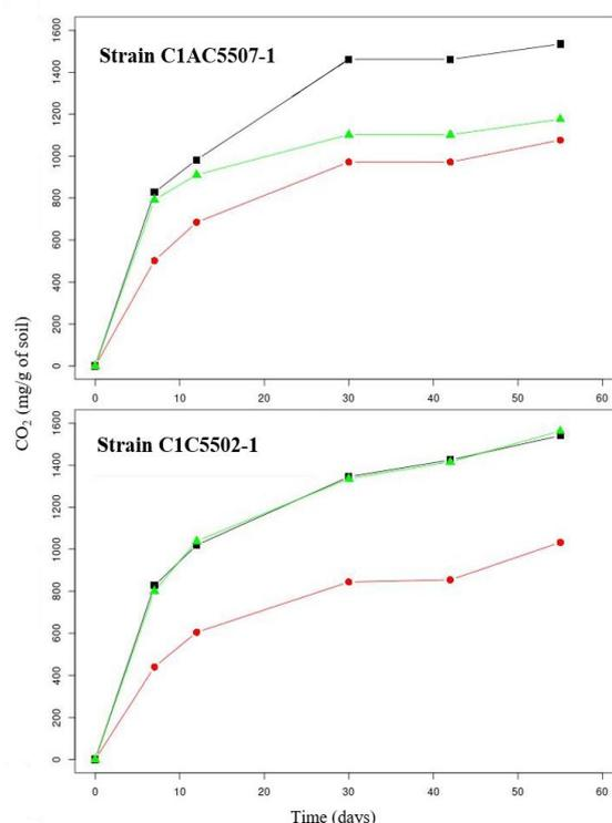
**Fig. 2.** Average cumulative CO<sub>2</sub> production by *Bacillus safensis* strains in HZN-contaminated reactors: Lipopeptide (black), fertilizer (red) and lipopeptide associated with fertilizer (green)
