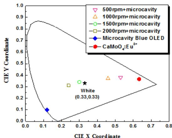
Figure 7: The CIE coordinates of WOLED driven at a current density of 20mA/cm<sup>2</sup>. A micro-cavity blue OLED is also indicated.
