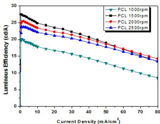
Figure 6: The dependence of luminous efficiency of WOLEDs on current density.
