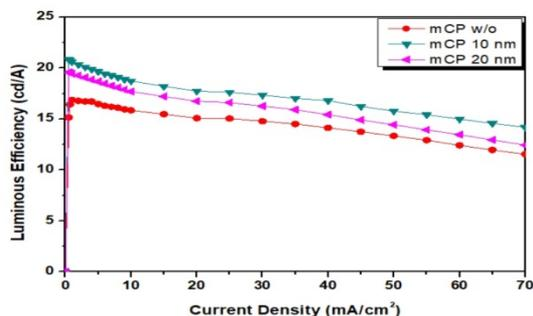
Figure 2: Luminous efficiency-current density characteristics of blue OLED.
