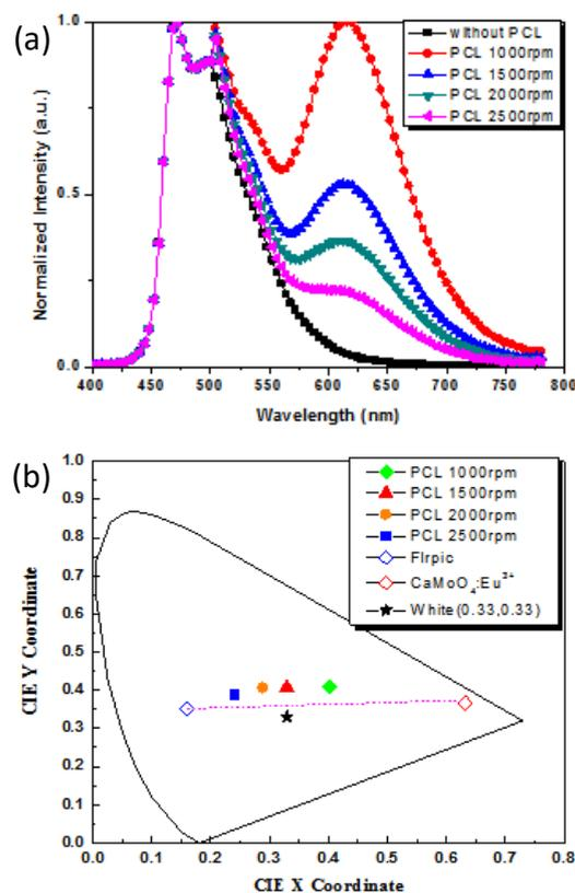
Figure 5: (a)The EL spectra of WOLED driven at 20mA/cm<sup>2</sup>, (b)CIE coordinates of WOLED driven at a current density of 20mA/cm<sup>2</sup>.
