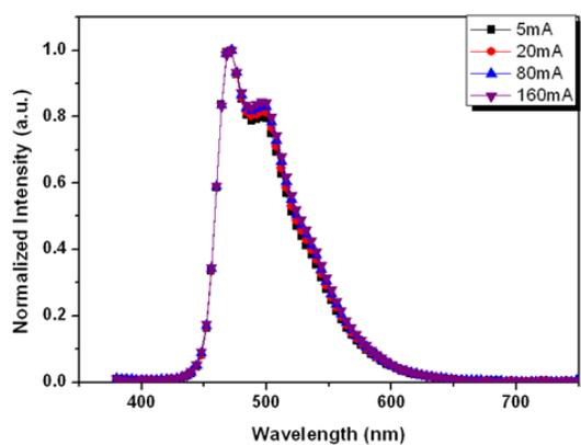
Figure 4: The EL spectra of blue OLED driven from 5 to 160 mA/cm<sup>2</sup>.
