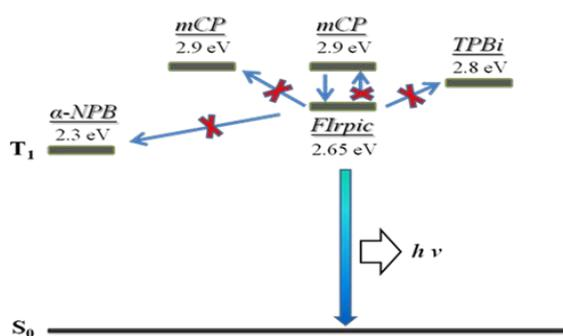
Figure 3: Triplet energy level diagram of blue OLED.
