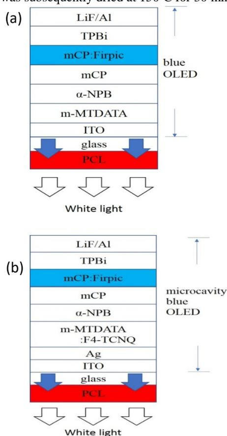
Figure 1: The WOLED architectures with (a) a blue OLED and PCL, (b) a micro-cavity blue OLED and PCL.
