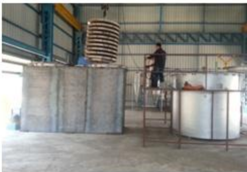
Fig. 1.1 – Loading & unloading the charge.
