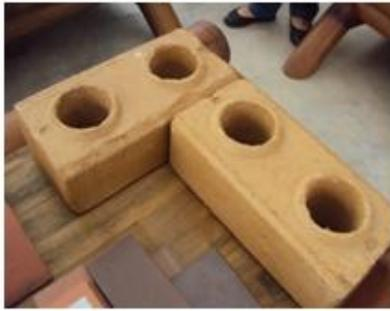
Picture 4. Soil Cement Block made with residual soil.
