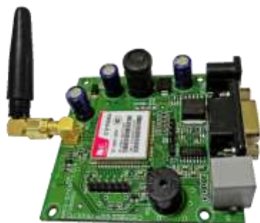
Figure 19. SIM900A GSM Module
