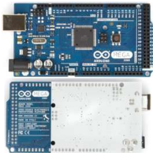
Figure 1. Arduino Mega 2560 Front and Rear Sections
