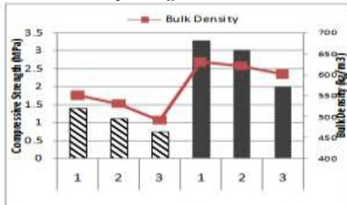
Fig. 4. Bulk density and compressive strength results.
