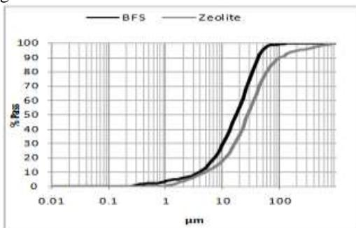
Fig. 1. Laser particle size analysis of zeolite and BFS
