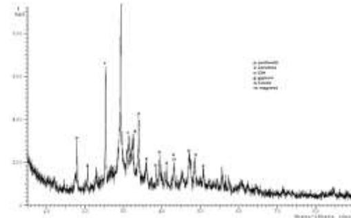
Fig. 5. XRD analysis of BFS samples
