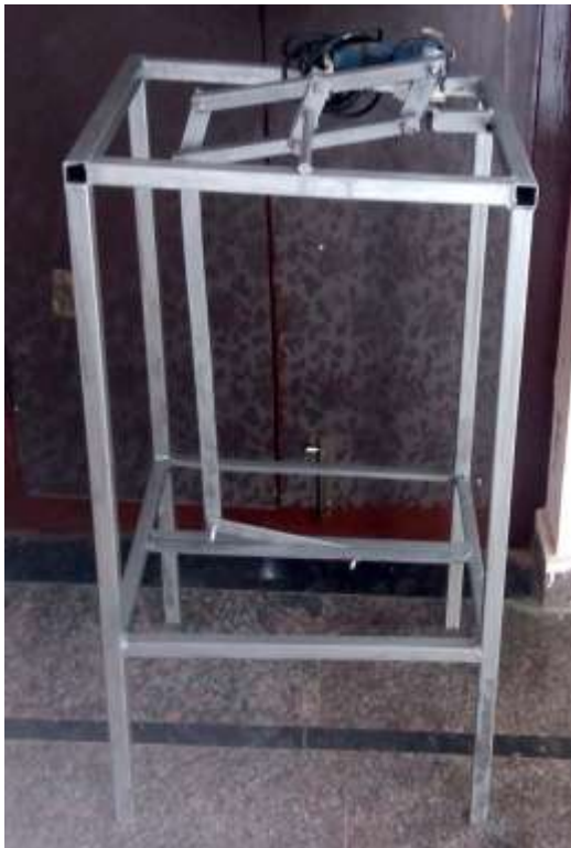
Fig 4.1 : Experimental setup of mechanical cutter.
