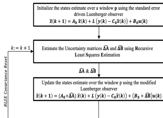
**Figure 2.** Flowchart of Computing the Parameter and State Estimate using Observer-RLSE-CR Method.
