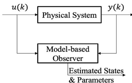
**Figure 1.** Block Diagram of the Physical System and the Observer.
