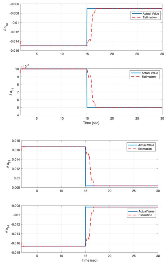
**Figure 11.** Estimated Elements of the  $\Delta A$  State Matrix using Observer-RLSE-CR Method.
