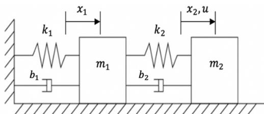
Figure 3. Double-Mass-Spring-Damper System.
