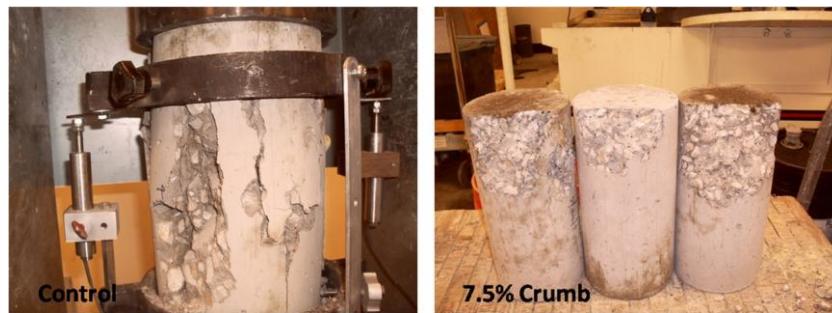
FIG. 4 —Fracture of control concrete and concrete with 7.5% fine aggregate replaced with crumb rubber. From the figure, it can be seen that the concrete with crumb rubber did not have cracks running through it.
