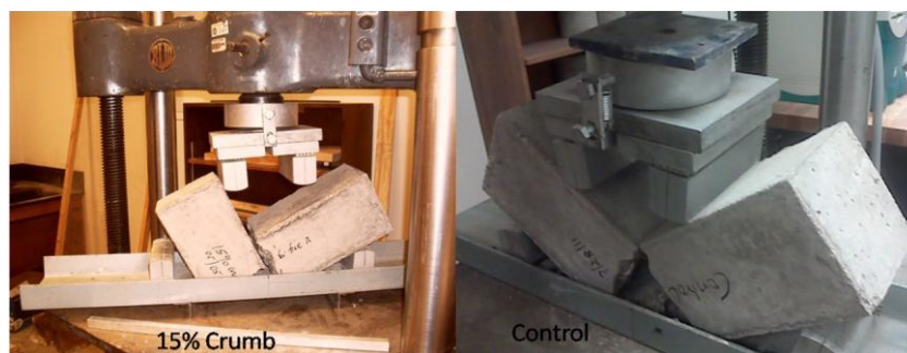
FIG. 13—Fracture pattern for control concrete and concrete with crumb rubber.
