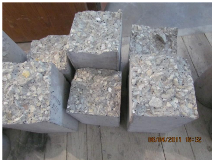
FIG. 5 —Distribution of crumb rubber in the concrete. The black spots represent crumb rubber.
