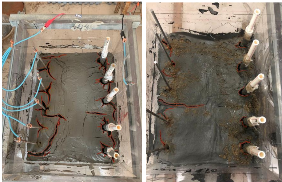
(a) T1 crack formation (b) M1 crack formation
