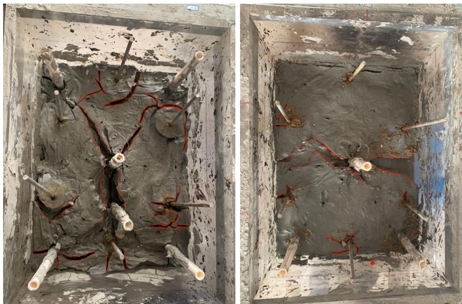
(a) T3 crack pattern (b) M3 crack pattern Figure 20. T3 and M3 crack pattern after experiments
