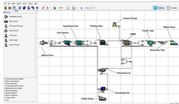
Fig. 2. Flow chart of Modified STP in GPS-X
