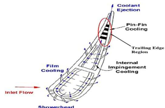
Fig 1.1: Sectional view of the blade [Courtesy: Google]
