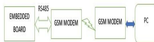
FIG NO. 3 : THE EMBLED SYSTEM'S BLOCK DIAGRAM WITH A BASIC DIVERSION DIAGRAM.
