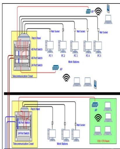
Fig 6– 24 and 48 port switch architectural design from server room to the whole floor
