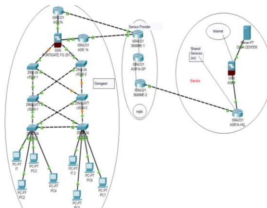
Fig 3- main site and branches interconnected design diagram
