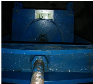
Figure 9 Uniform Pressure Applied on Brick
