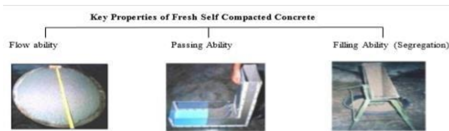
Fig 1: Key properties of fresh self-compacted concrete
