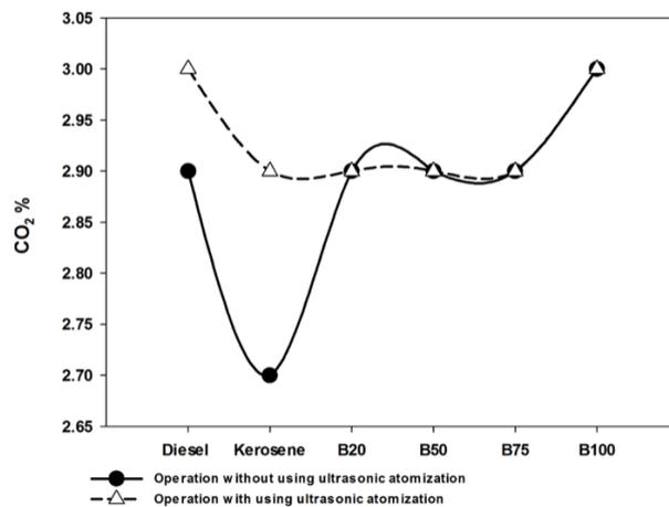
**Figure 4.6: Plots of CO<sub>2</sub> emission against the engine load for all the different fuel type at maximum load thrust force.**
