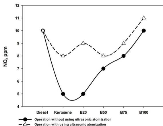
**Figure 4.10:** Plots of NO<sub>2</sub> emission against the engine load for all the different fuel type at low load thrust force.
