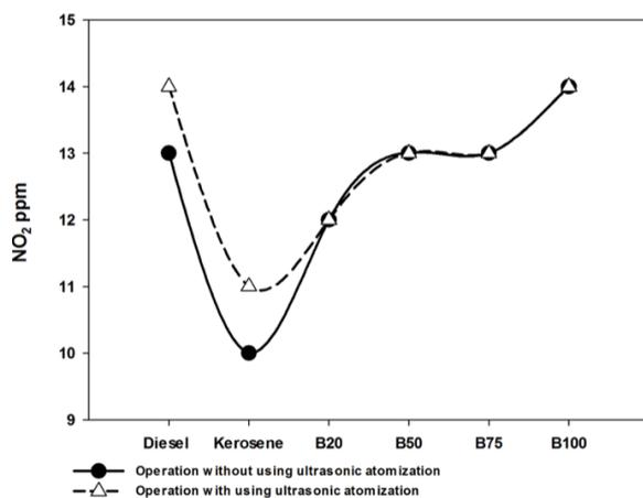
**Figure 4.11:** Plots of NO<sub>2</sub> emission against the engine load for all the different fuel type at medium load thrust force.
