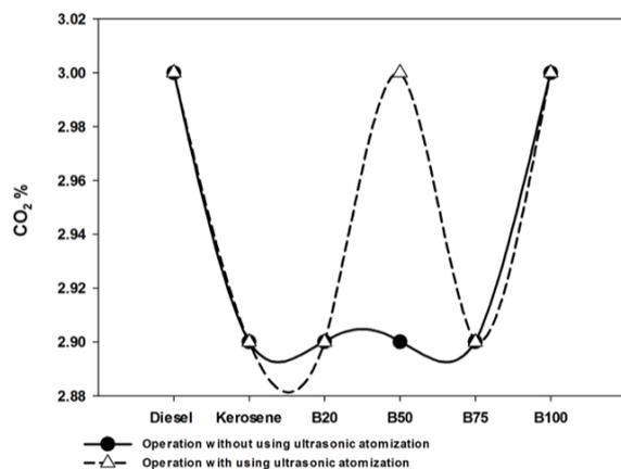
**Figure 4.4: Plots of CO<sub>2</sub> emission against the engine load for all the different fuel type at low load thrust force.**
