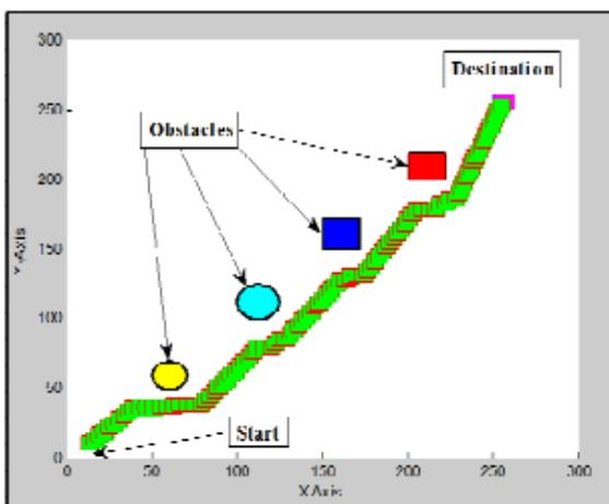
Figure 6: Navigation path for obstacles avoidance of mobile robot using fuzzy controller
