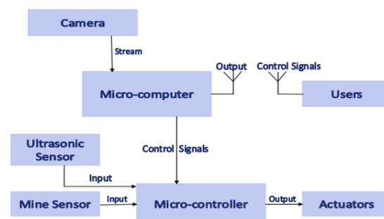
Fig 1: Block Diagram of the Robot
