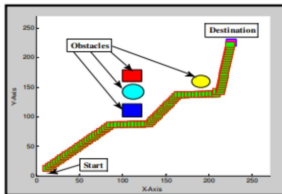
Figure 7: Navigation path for obstacles avoidance of mobile robot using fuzzy controller.
