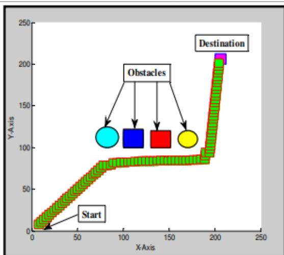
Figure 5: Navigation path for obstacles avoidance of mobile robot using fuzzy controller.
