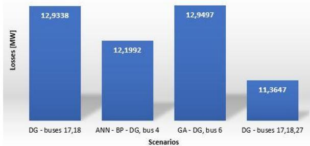
Fig. 5 Best scenarios for ANN with the insertion of Distributed Generators.
