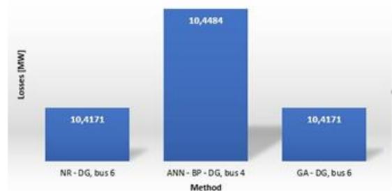
Fig. 2 Comparison between the methods applied to the IEEE-6 bus system.
