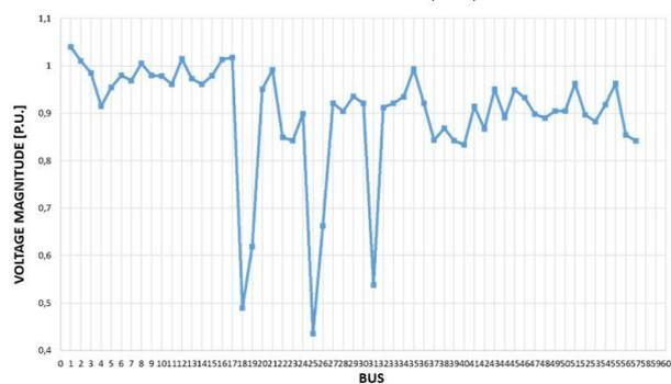
Fig. 8 Voltage Magnitudes for the IEEE-57 system without DG insertion.
