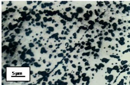
Fig. 3 Microstructure of compacted sample from Al-11%Si-0,022%Sr
