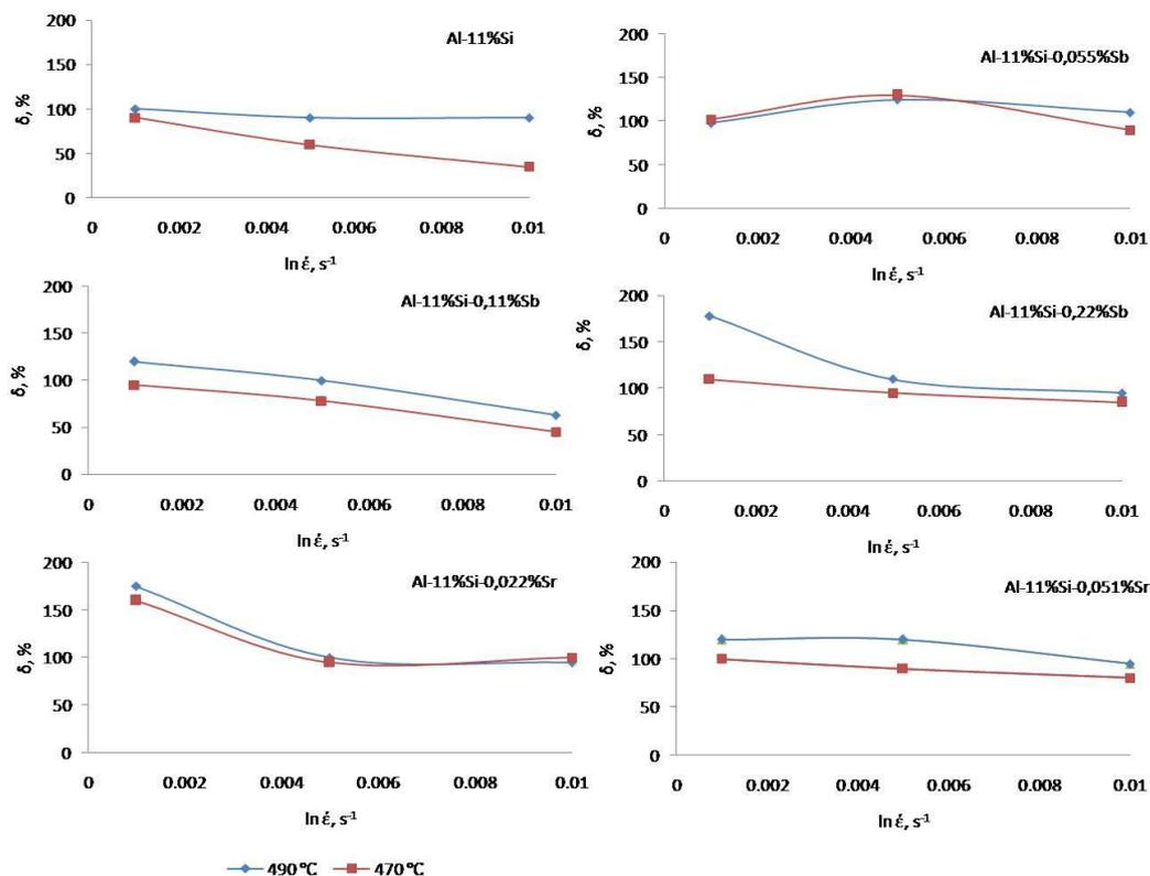
Fig.4 The dependence of the relative elongation on the deformation velocity and the temperature at high temperature deformation tests for all tested alloys.
