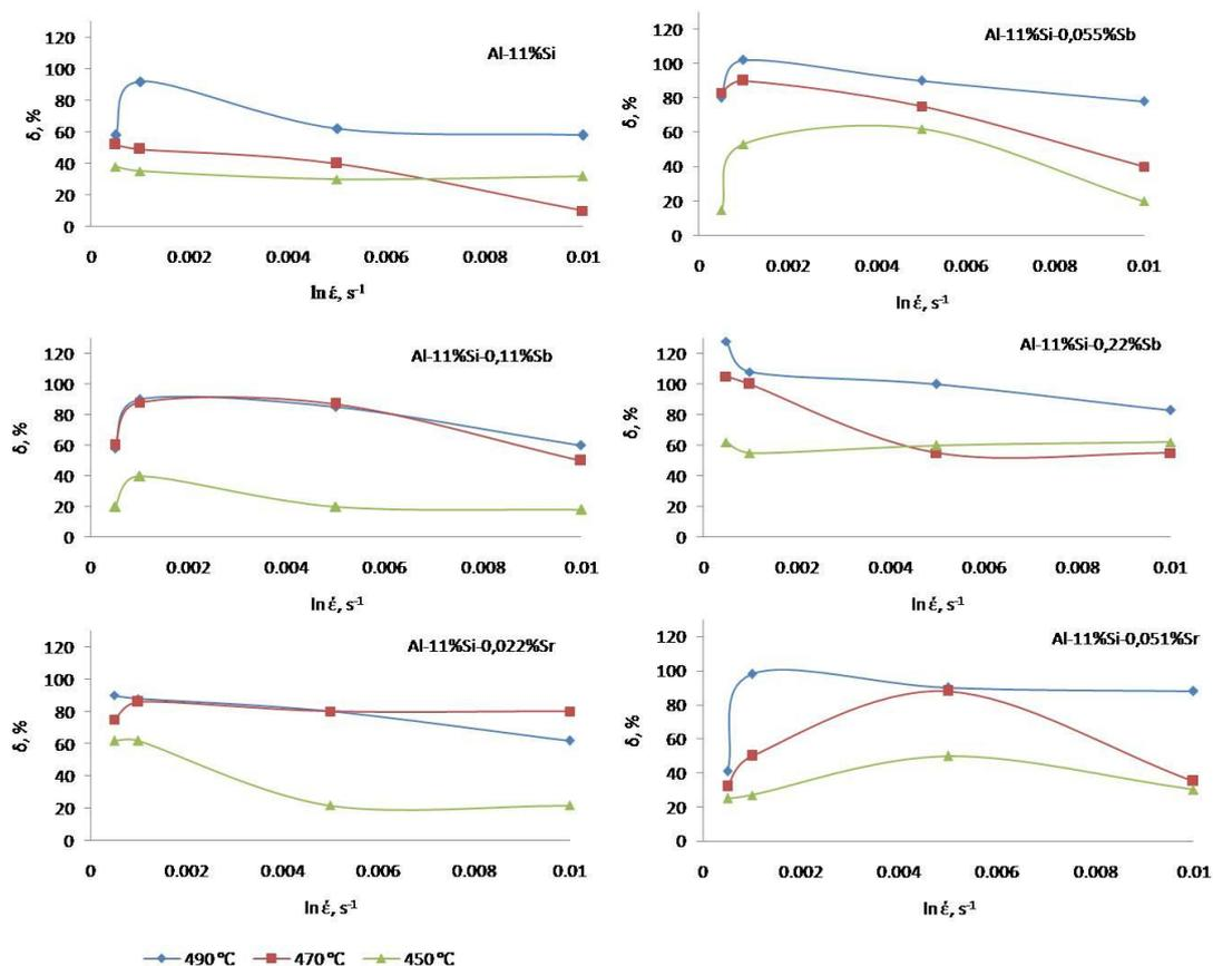
Fig. 2 The dependence of the relative elongation on the deformation velocity and the temperature.
