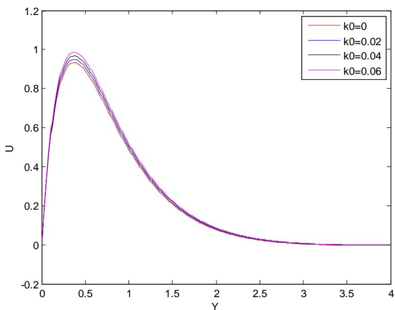
**Fig.2** Effect of chemical reaction parameter over velocity field
