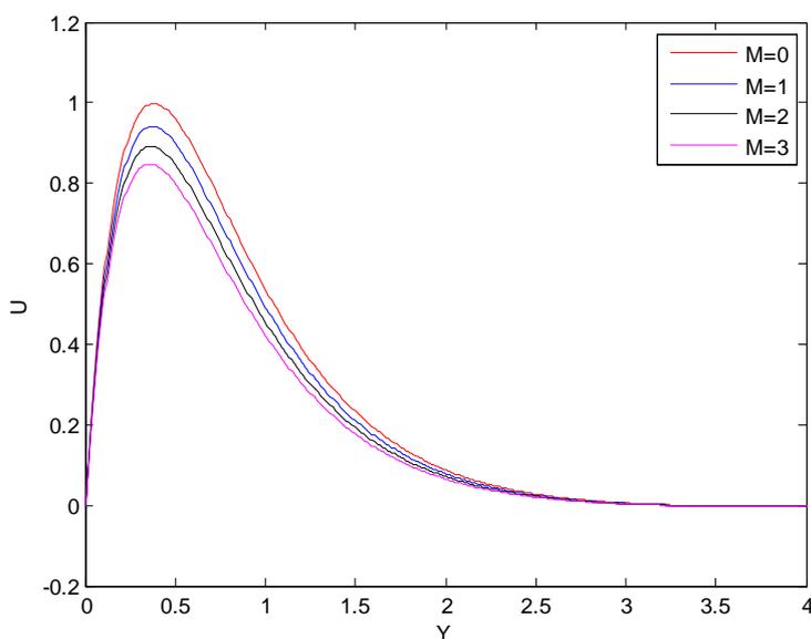
**Fig.5** Effect of magnetic parameter over velocity field
