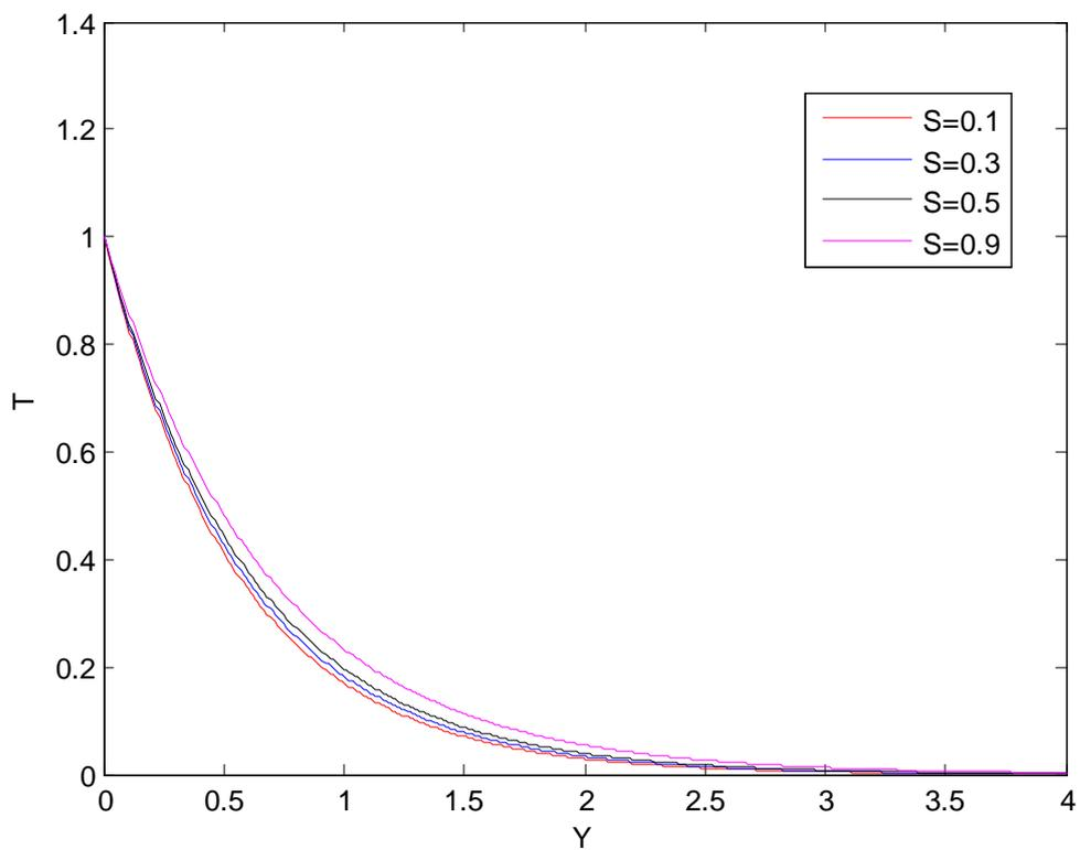
Fig.7 Effect of Heat source parameter over temperature field
