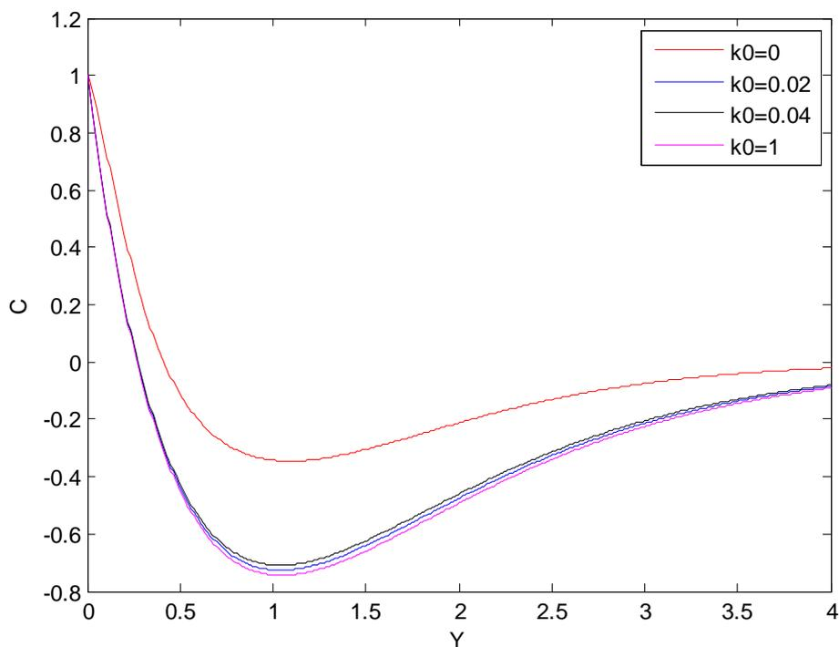
**Fig.1** Effect of permeable parameter over concentration field
