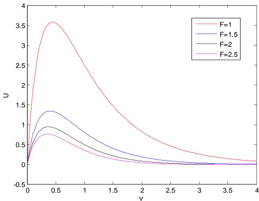
**Fig.4** Effect of radiation parameter over velocity field
