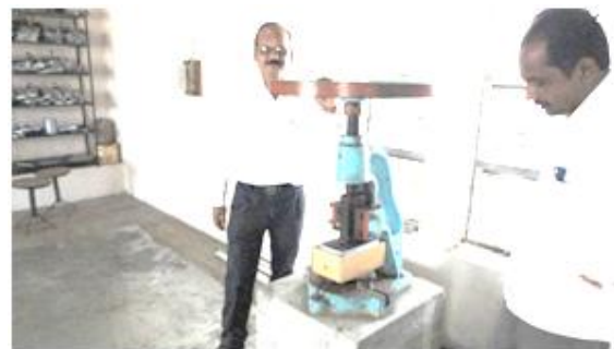
Figure 3: Compaction of soil sample
