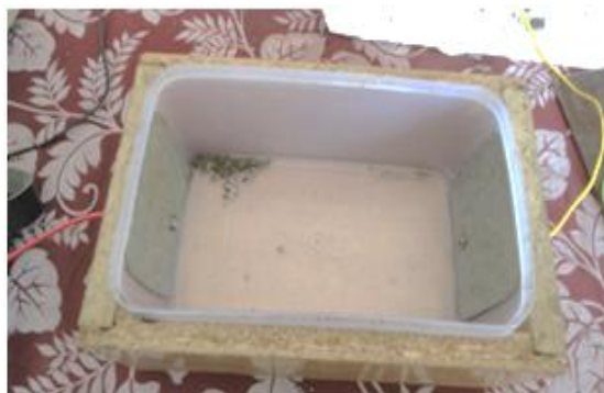
Figure 2: Test box for soil resistivity measurement
