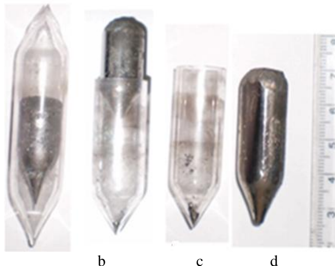
Figure-2 the sequence of the taking out ingot from ampoule, the as grown detached ingot were grown by VDS-process, a) As grown entire detached Sb-based ingot, b) Ingot taking out from an ampoule, c) The empty ampoule, d) The grown ingot and its surface features.
