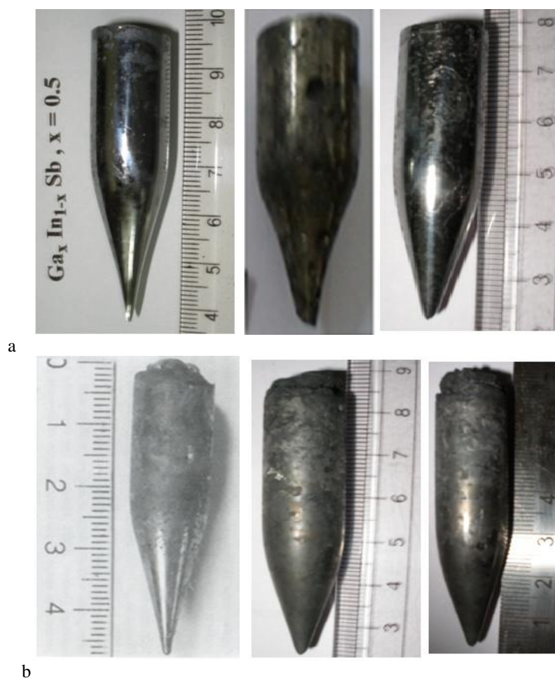
Figure-3 The as grown ingots of \text{In}_{0.5}\text{Ga}_{0.5}\text{Sb} , a) IGS-1, b) IGS-2, c) IGS-3, d) IGS-4, e) IGS-5, f) IGS-6
