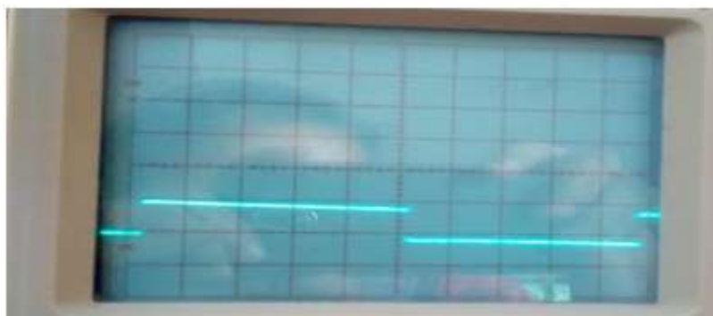
Figure 5.8 Gate pulses for switches S5 & S6
