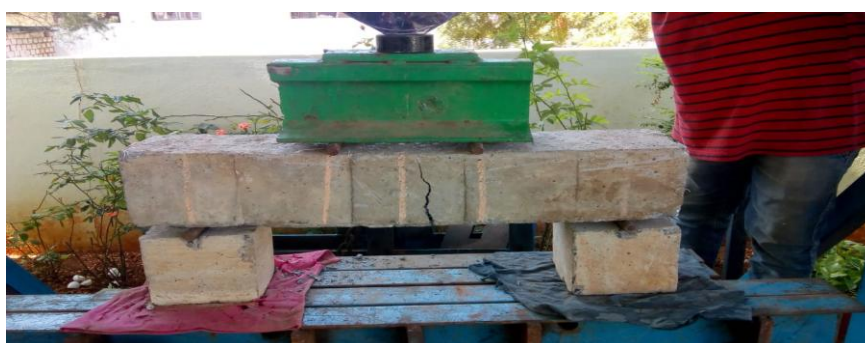
Figure 9. Two point loading setup for flexure test
