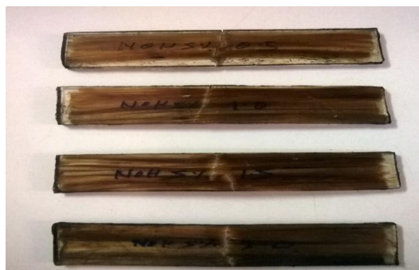
Fig 8 : Specimens of Hemp fiber polyester composite after flexural testing
