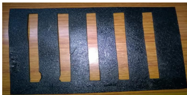
Fig 3: Die for making tensile testing specimens
