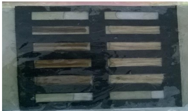
Fig 5: Die for making bending/flexural testing specimens
