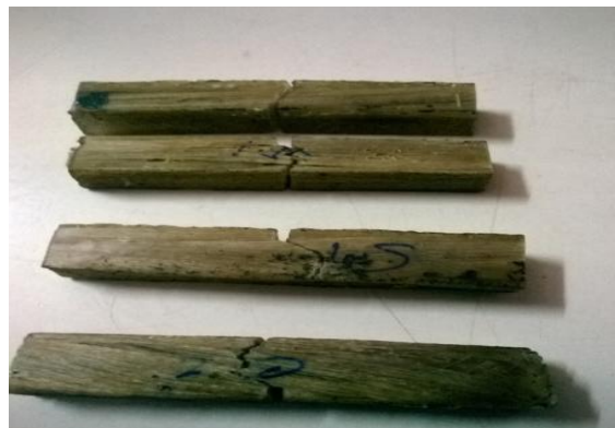
Fig 7: Specimens of Hemp fiber polyester composite after impact testing
