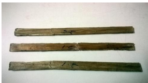
Fig 6: Specimens of Hemp fiber polyester composite after tensile testing
