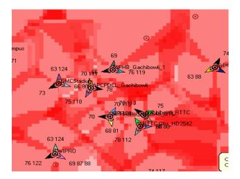
Fig.7. Removed interference zones in automatic frequency planning
