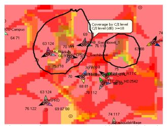
Fig. 6.Interference zones occurred in manual planning
