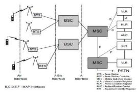
Fig .1. Outline of GSM network architecture
