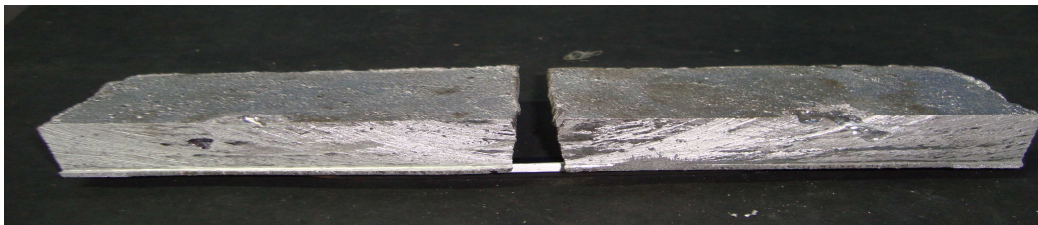
Fig3(b) Sample with Riser Ø 36mmx72mm Height with Neck Ø 20mmx5mmHeight
